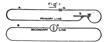
A is the primary line; a, the battery; b, the key. B is the secondary line in which is placed the galvanometer c.
